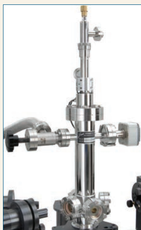
Cryostat (4.2K to 500°C)
