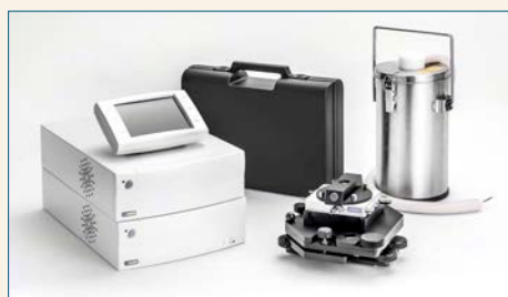
Variable Temperature Stage (-70°C to 600°C)
