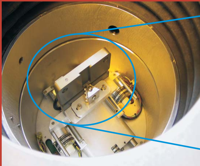
Figure 2. Liquid prism cell attached to VUV-VASE sample stage. The hollow stainless steel prism can be fitted with windows of either fused silica or calcium fluoride.
