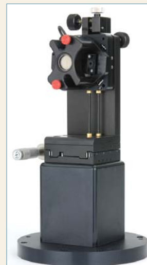
270µL Vertical Liquid Cell
