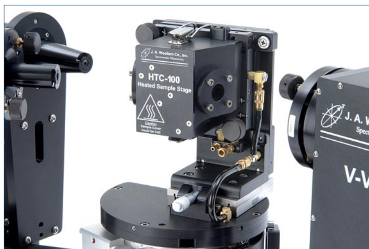
Figure 3. VASE ellipsometer with heating cell option attached.
